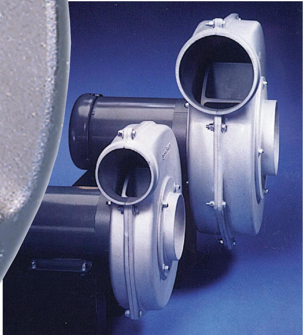
Chicago castings blend aluminum with high-strength alloys to create strong, corrosion-free housings and wheels ideal for adverse industrial environments. Aluminum also stands up to sub-zero ambients without material deterioration. Since aluminum is non-magnetic and non-toxic, Chicago's pressure blowers are recommended for both electronic and food related applications. The non-sparking properties qualify Chicago's pressure blowers for AMCA Type B spark resistant rating.
