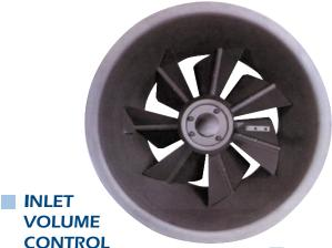
When the fan is used for varying or partial load applications, the Inlet Volume Control (IVC) provides precise air control and more efficient operation. Adjustable guide vanes pre-spin the incoming air in the same rotation as the wheel to produce the desired volume of air at the exact pressure.
