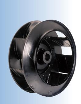
Chicago Blower's wheels feature airfoil blades continuously welded to a streamlined wheel cone and heavy steel backplate. The hollow blades have weep holes to prevent moisture build-up inside the blade.
