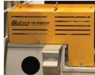
Typical Options include Manual Inlet Volume Control, Inlet Screen and Raised Access Door.
