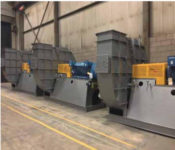
*Three Design 5500 Size 6000 Arrangement 8S PBC fans with raised access door, split housing, and fan bearing RTDs for a combustion air application.*
