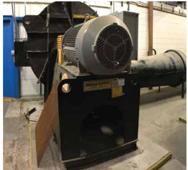
*A Size 4014 Arrangement 8S PBC Design 5800 fan with split housing, being used in a glass tempering application.*
