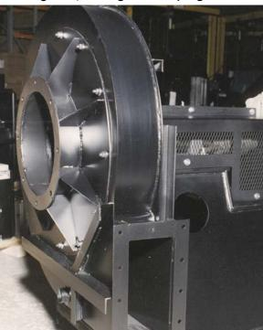
An unpainted fan showing continuous housing welds, stiffener stitch welds and plug welds for scroll and side liners
