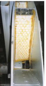
Ceramic lined blades extend wheel life in abrasive applications
